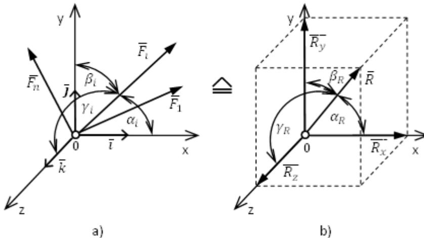
In a rectangular coordinate system  $0, x, y, z$ , the resultant  $\underline{R}$  can be divided into the components
