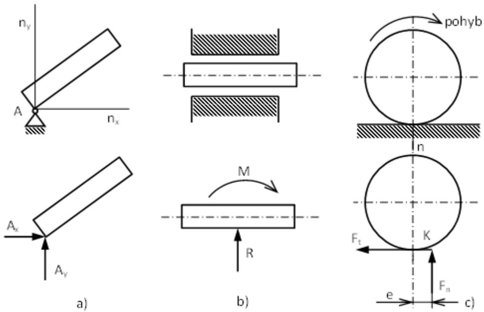
A particle can be rigidly fixed with other particle, e.g. with a frame by means of so-called restraint (Figure 3.7), which removes all three degrees of freedom of movement from the particle in the plane.
