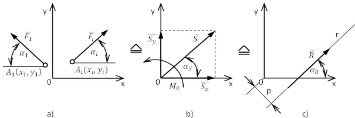
General planar force system consists of forces distributed in the plane (e.g. in plane  $x, y$  shown in Figure a). The effect of each force  $\underline{F}$  at the beginning of a coordinate system  $0, x, y$  will be both sliding  $\underline{F}_i$  and rotational  $\underline{M}_{i0}$ . The resulting sliding and rotational effect of the force system to the starting point in point  $0$  will be (Figure ):
