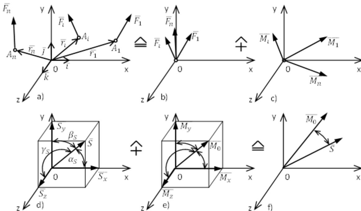
The angle  $\varphi$  (Figure f) can be determined by means of scalar product
