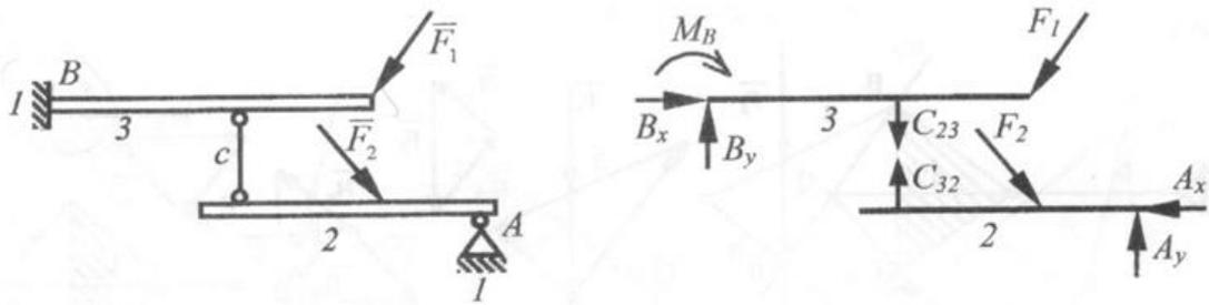
Based on the body 2 equilibrium,  $A_x$ ,  $A_y$ ,  $C_{32} = C_{23}$  will be determined; based on the body 3 equilibrium,  $B_x$ ,  $B_y$ ,  $M_B$  can be calculated.
