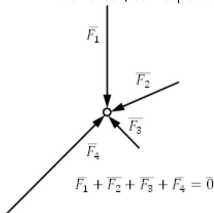
For CPFS only two static conditions can be written from which we can calculate two unknown parameters.
