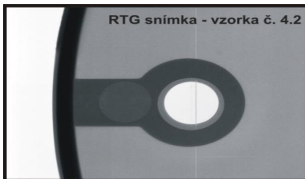
Fig. 15 X-ray image sample No. 4.2, v = 2.9 \text{ m.s}^{-1} \text{m.s}^{-1}
