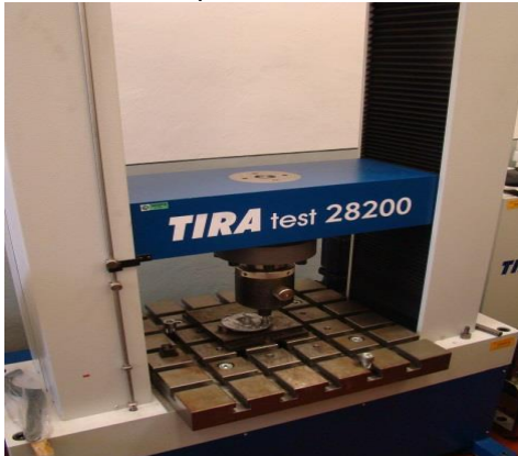
Fig. 11 Measuring equipment TIRAtest 28200 the casting
