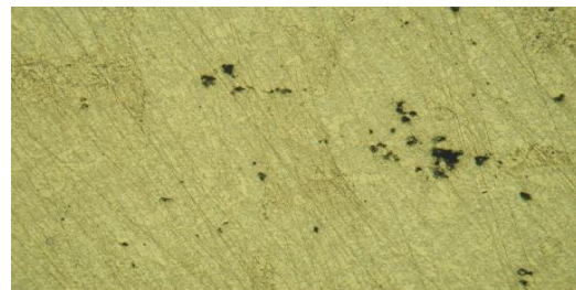
Fig. 32 Porosity 0.85 % p = 25 \text{ MPa}
