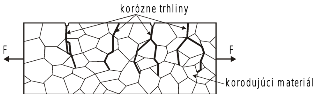
Figure 7.3 Corrosion cracking scheme
