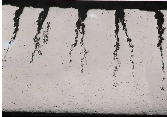
Figure 7.4 Microphotograph of corrosion cracking
